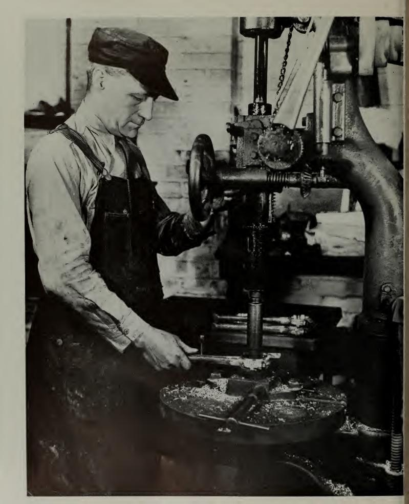
The outer edge of the babbitt flange is now faced by a special tool placed in a drill press. Approximately 50% of the rods rebabbitted were of a type that required this operation, which is shown in the above picture.
